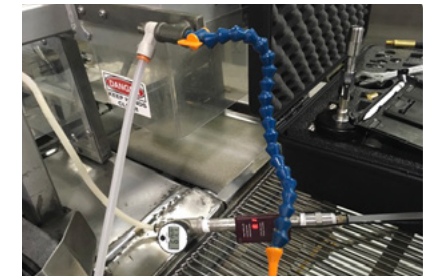
The Henderson bakery also removed energy waste from its compressed air system by redesigning air nozzles.
