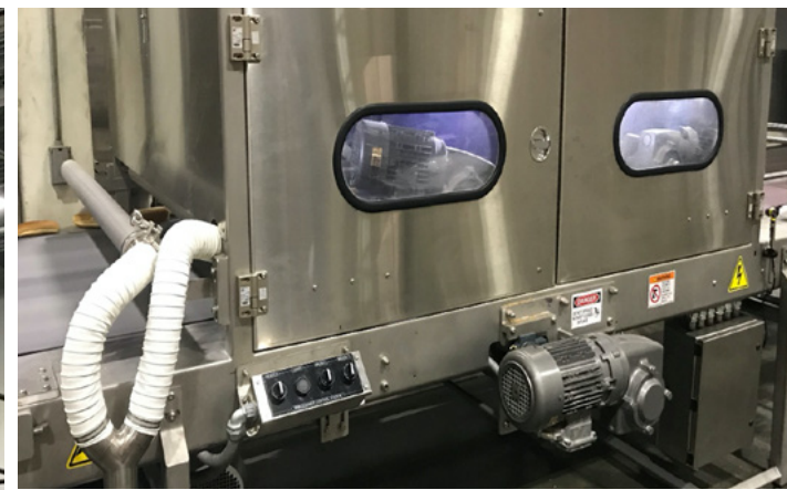
The line’s new pan cleaner uses an electric blower rather than compressed air to improve energy efficiency.
